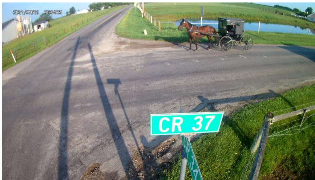
Figure 3. Typical stopping location of a horse-drawn vehicle on minor road approach
