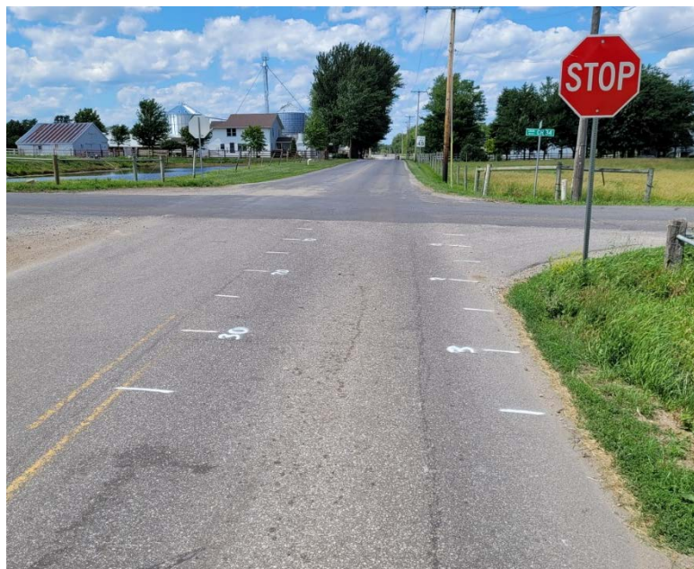
Figure 2. Intersection of CR 34 and CR 37 showing pavement markings used for determination of vehicle stopping position
