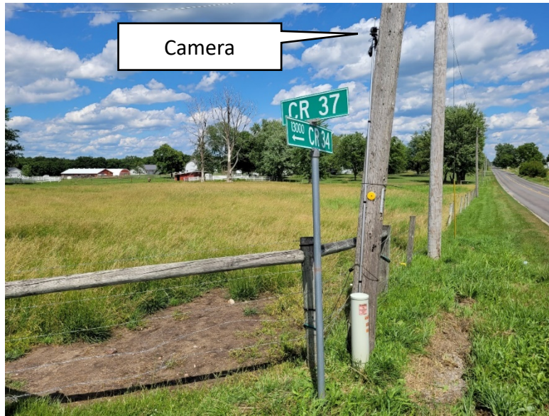
Figure 1. Typical camera placement at intersection corner
